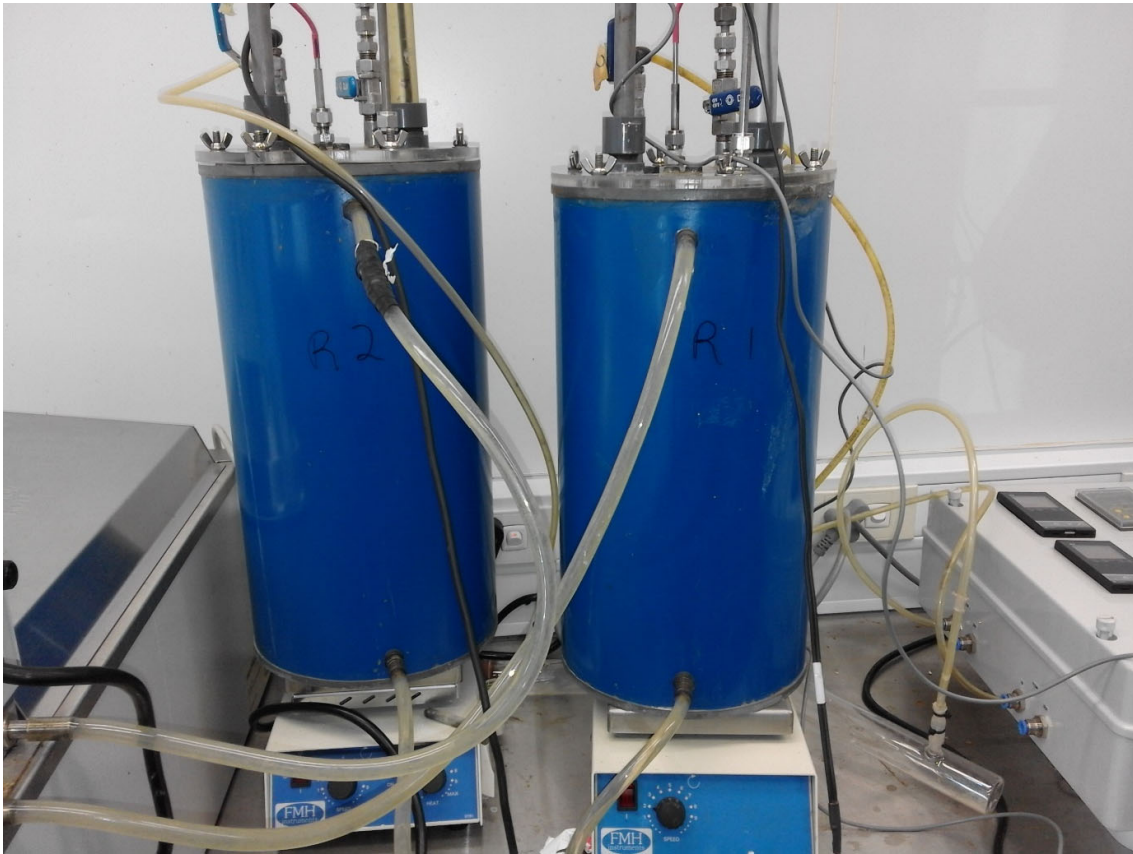
Figure 0-6: shows two 6.5 L batch reactors for screening industrial wastewater
