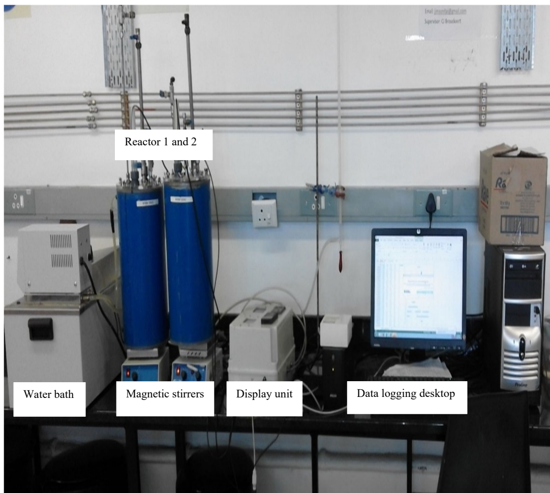
Figure 0-31: Laboratory screening equipment showing two batch reactors connected to a water bath, pH probes, temperature probes, gas flow meters and a desktop for data logging
