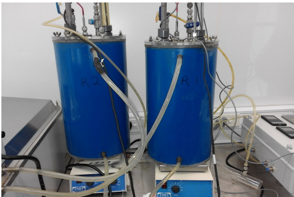
Figure 0-25: Laboratory screening batch reactor one and two, both with pH, temperature probes at the top and magnetic stirrers at the bottom. The reactors also have airtight transparent lids at the top.
